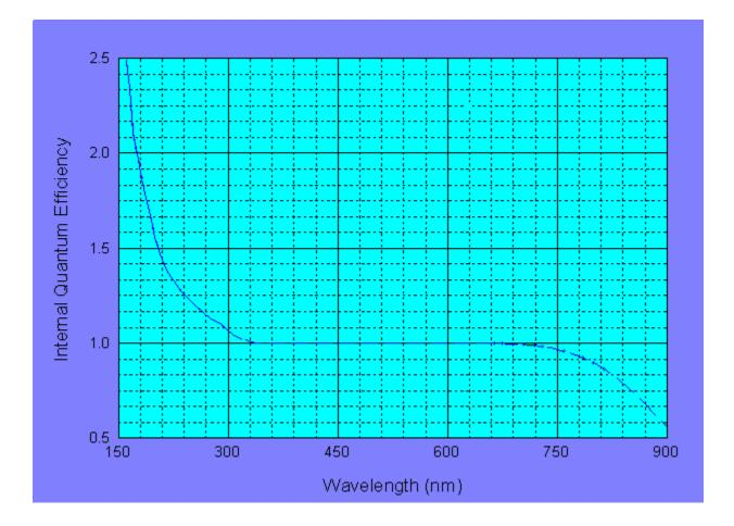
Fig. 1: Internal quantum efficiency of UVG photodiodes
