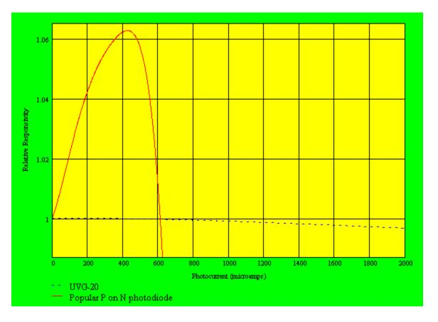
Fig. 3: Linearity of UVG-20 photodiode and widely used P-on-N photodiode when tested at 980 nm with no reverse bias
