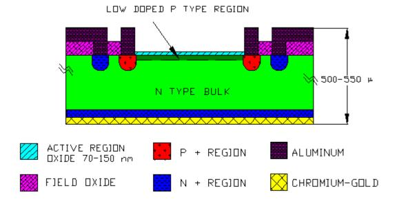
Fig. 4: Structure of the UVG-PN20 photodiode
