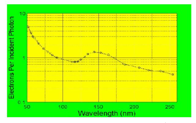
**Fig. 1:** Quantum efficiency of UV-enhanced photodiodes with 60 Å oxynitride passivating front window. O Before exposure, X after exposure to 100% relative humidity for 4 weeks.
