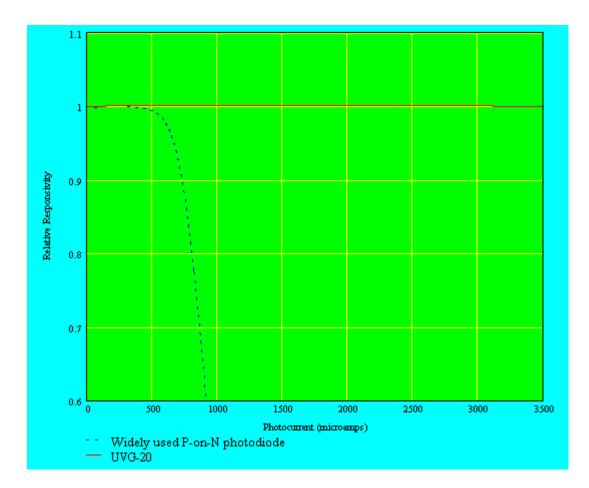
Fig. 1: Linearity of UVG-20 photodiode and a widely used P-on-N photodiode when tested at 430 nm with no reverse bias.
