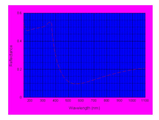
Fig. 2: Typical reflectance of UVG series photodiodes.
