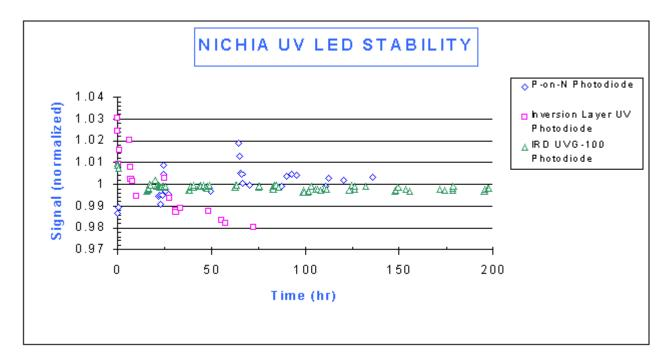
Fig. 4: Nichia 378 nm LED stability measured with p-on-n, inversion layer, and the UVG-100 photodiodes [7].
