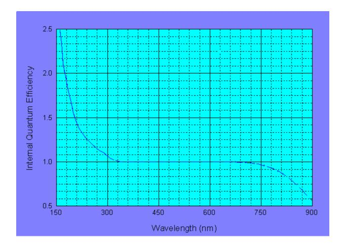
Fig. 1: Internal quantum efficiency of UVG photodiodes
